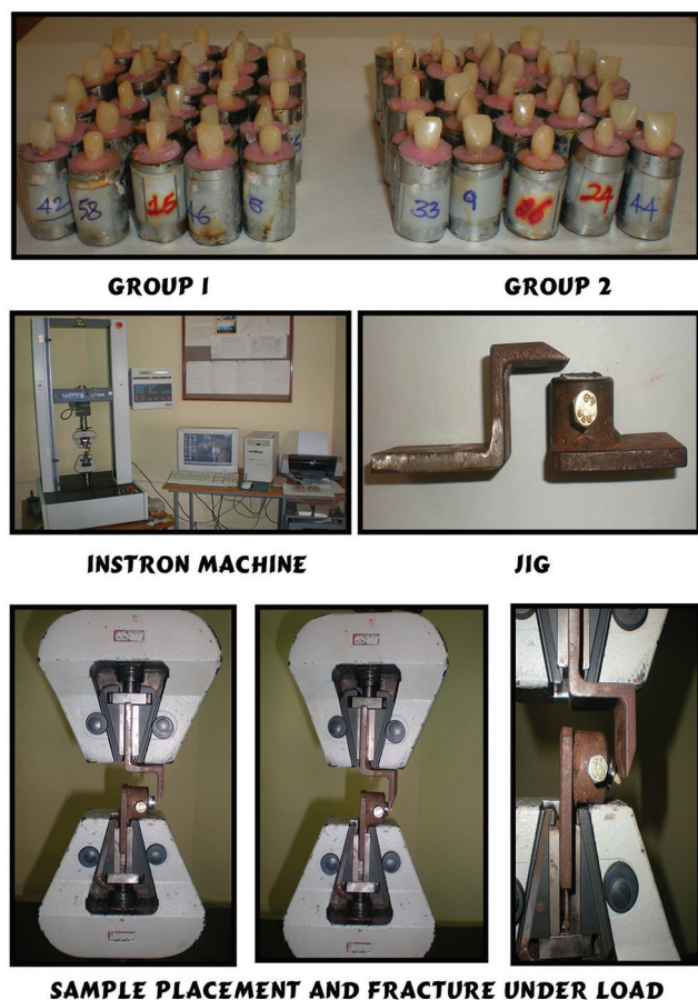
Figure 3: Fracture resistance test using the Instron machine.
