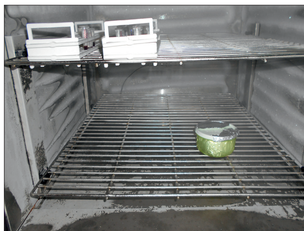
Figure 2: Storage of Head Cured polymethylmethacrylate resin at Dough stage in Deep Freezer
