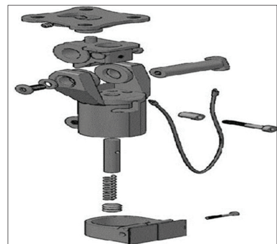
Figure 2: Assembly drawing of safe gait prosthetic knee joint
